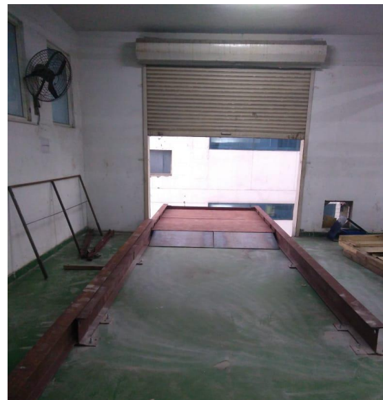
Fig 2. Inside view of the setup of rail guides for moving machine
